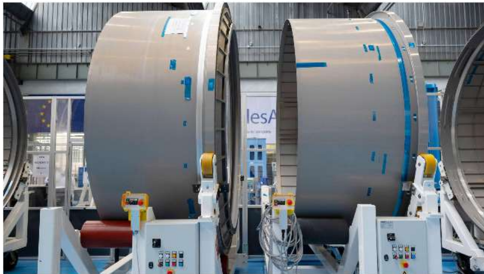
Gateway's Lunar I-Hab module under construction at a Thales Alenia Space industrial plant in Turin, Italy.
